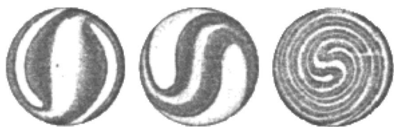
Figure 2. Drawings by Lehmann of typical cholesteric droplets continuously rotating anticlockwise when heated below (reproduced with permission from (1)).
